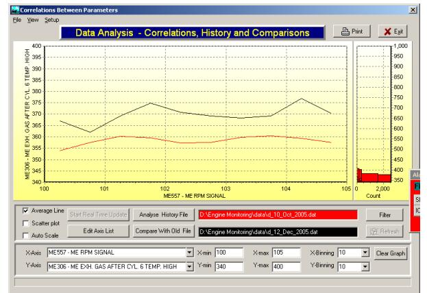
Fig. 10: Mean exhaust gas temp, filtered by draught.
