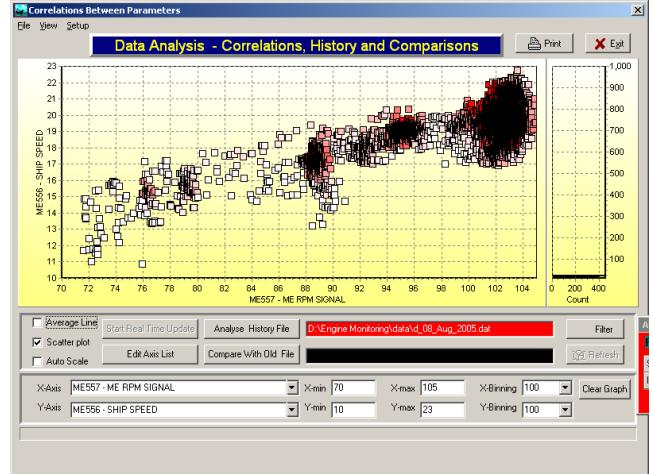
Fig. 3: Speed vs. RPM, no Filter
