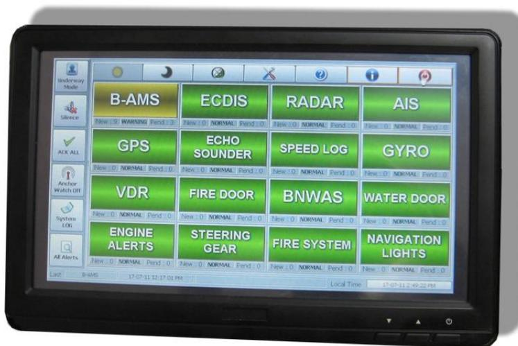
The main backbone of the BAMS is the interface to all relevant bridge systems, either through serial inputs using NMEA protocol or alternately through hard wire (binary) signals. The BAMS shows all the systems in a clear display on a touch screen monitor, allowing fast identification of the faulty system and rapid silencing of the audible signal. The cause of the alarm can be seen in a clear way using the information transmitted by the faulty system.
