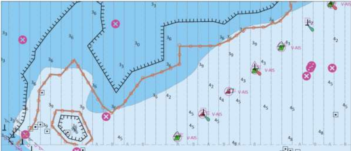
Two automatically created 'no-go' areas. Source: ECDIS Procedures Guide 2024 - 2025 by Witherbys
