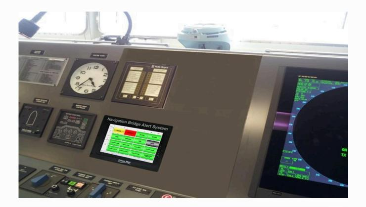
Approved as per: IEC62923:2018 - Bridge Alert Management Standard, MSC.128(75)- Performance Standard for Bridge Navigational Watch Alarm System.
